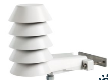
HMS110 Outdoor Humidity and Temperature Transmitter Accuracy \pm 2\% RH, \pm 0.2^\circ\text{C} ( \pm 0.36^\circ\text{F} ) Outputs: 4-20 mA, Modbus RTU Integrated rain / solar radiation shield Tolerant of high winds and icing conditions
