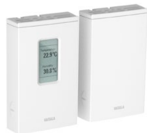
HMW90 Room Humidity and Temperature Transmitter Accuracy \pm 1.7\% RH, \pm 0.2^\circ\text{C} ( \pm 0.36^\circ\text{F} ) Outputs: 4-20 mA, 0-10 V, Modbus RTU Exchangeable measurement modules Display with sliding cover
