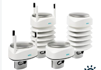
WXT530 Weather Transmitter Weather parameters: air pressure, temperature, humidity, rainfall, wind speed, wind direction Output: Modbus RTU Integrated radiation shield
