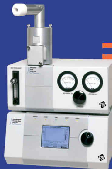
The Impactor Inlet 3306 is designed to sit atop the Aerodynamic Particle Sizer™ spectrometer model 3321.
