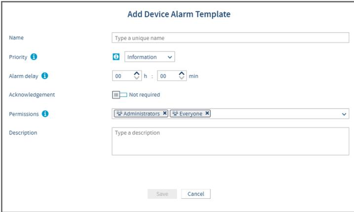
3. In the **Add Device Alarm Template** window, type a unique name for the new template and then set the template properties:
