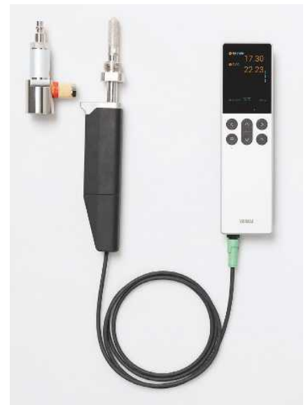
Vaisala Indigo80 indicator combined with DMP80 handheld probe and DSC74 sample cell.
