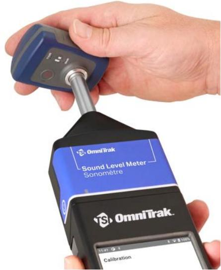
**Figure 3-7. Calibrator Attachment**
