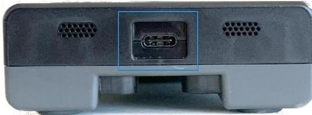
**Figure 1-2. Smart Station USB-C port**
