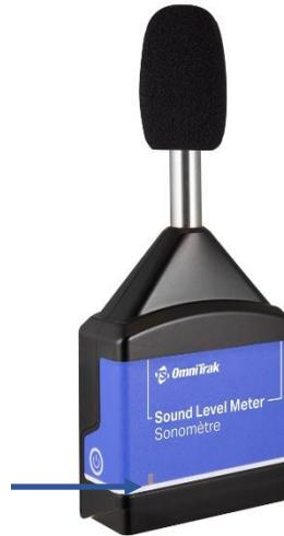
**Figure 2-7. SLM Module Connection Indicator**
