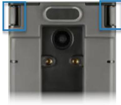
Figure 2-9. Smart Station latch releases
