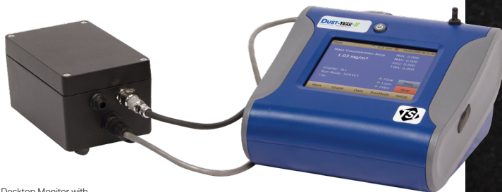
Desktop Monitor with External Pump, Model 8530EP
