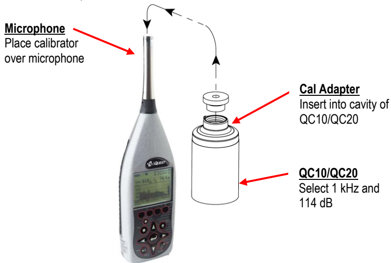
Figure 5-2: Attaching calibrator to SoundPro
