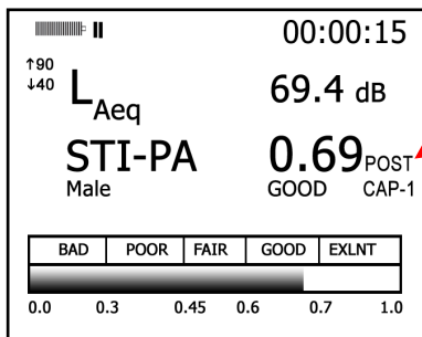
Figure 6-27: Post CAP-1 applied during STI-PA test
