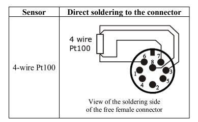
4 wire Pt100 sensors can be soldered directly to the pins of the free female connector without making use of the TP47 board. The 4 wires of the Pt100 sensors have to be soldered as indicated in the figure on the left.
