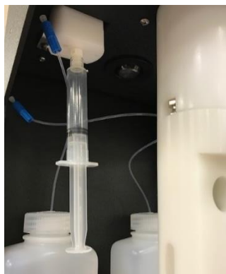
Figure 13 – Pump Priming with Accessory Syringe
