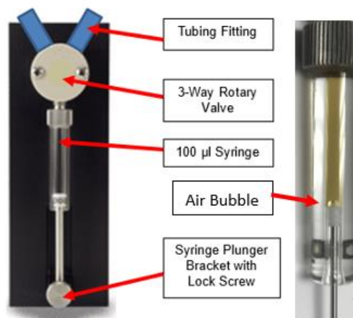
Figure 6 – Syringe Pump Components
