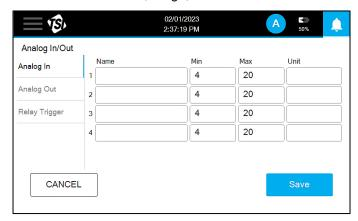
Select the particle size data and scale to be communicated out through the analog outputs on the **Analog Out** screen.
