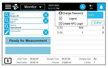
A prompt will appear. Hold an NFC card near the NFC Reader/Writer. The prompt will be dismissed and a beep will sound to indicate the card has been programmed.
