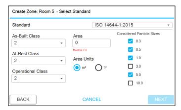
Select the class(es) for all occupancy states; the enabled Considered Particle Sizes will update to all those specified for the class(es) selected. Disable or enable the desired Considered Particle Sizes. Enter the area of the zone. Press the **NEXT** button.
