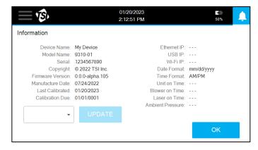
Firmware updates can be performed by inserting a USB drive with updated version of the firmware into the USB port. The list of available versions will appear in the drop-down. Select the desired version and press the **UPDATE** button. Firmware is downloaded from the TSI® website.
