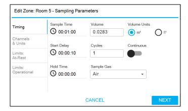
The parameters on the Timing screen are described in detail in Manual Mode. The Channels & Units screen is used to select the particle sizes that will be displayed. The Units for Limits can be selected from the drop-down. Alert and Action limits can be entered for enabled sizes on the Limits: At-Rest and Limits: Operational screens. Press the **NEXT** button to add locations.
