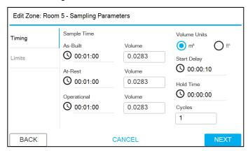
The parameters on the Timing screen are described in detail in <u>Manual Mode</u>. The sample times and volumes will default to the minimum required per the selected class(es). The limits will autopopulate with the limits for the selected standard. Press the **NEXT** button to add locations.
