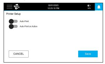
Turning on **Auto-Print** will automatically print the sample record at the end of sampling. Turning on **Auto-Print on Action** will automatically print the sample record at the end of sampling only if the action limit was exceeded.
