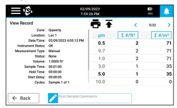
The columns in the results table are selectable by pressing on the box at the top of the column. A comment can be added to the record by entering it in the **Post Sample Comments** field at the bottom of the screen. Press the **Printer** icon to print the record with the thermal printer. The arrow buttons can be used to scroll through records.
