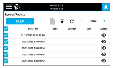
Records are listed with the most recent on top. Press the arrow buttons, 1/2132 >, to scroll through additional pages of records. If actively sampling, press the **Refresh** icon **C** to refresh the list and add any new records that have completed since the list was previously generated.
