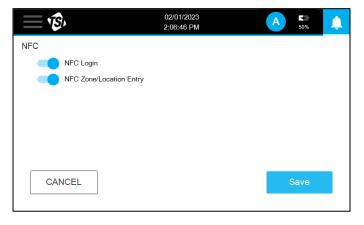
With NFC Zone/Location Entry turned on, an NFC card can be programmed by going the Sample screen in either Monitor or Classify mode. Select a Zone and Location and tap the 🗓 icon. A prompt will appear.
