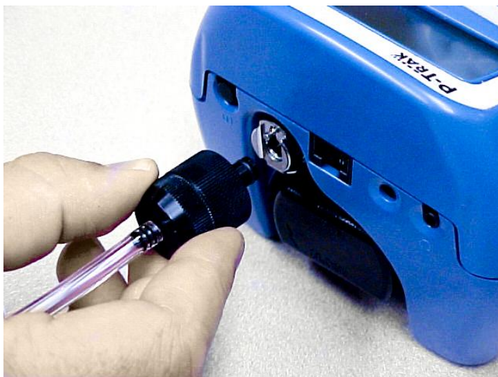
Figure 2-7: Insert Inlet Screen Assembly into Fitting
