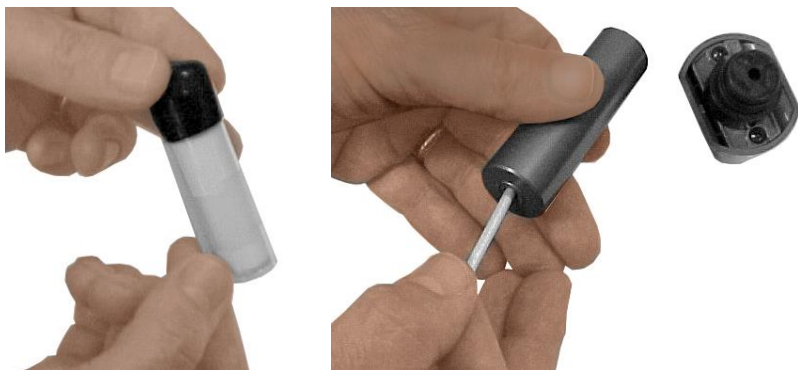
Figure 4-2: Remove Wick and Screen Using Dowel
