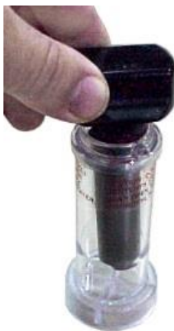
Figure 2-5: Insert Alcohol Cartridge into Fill Capsule
