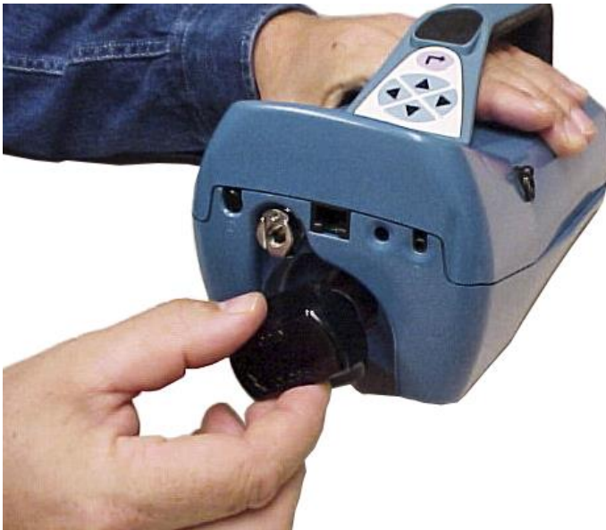
Figure 2-6: Insert Alcohol Cartridge into P-Trak Particle Counter
