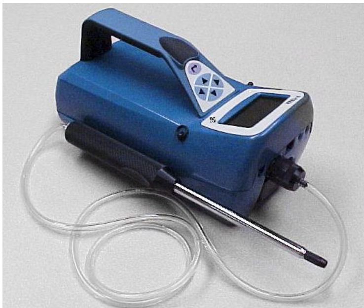
Figure 2-8: Slide Telescoping Probe onto Instrument Case
