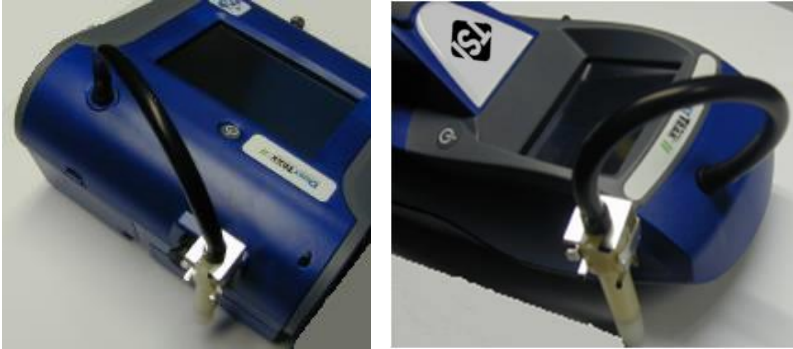
Figure 2-8: Installing Door-Oliver Cyclone
