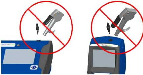
Figure 4-3: DO NOT Blow into Instrument
