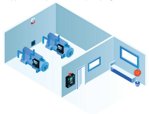
chillers in the room, a CGAS-D-IR transmitter should mounted as close as possible to each potential leak point.
