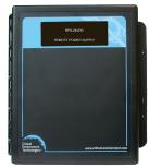
The RPS-24VDC is a remote power supply for large fixed system applications and/or very long wire runs. It converts 90 - 240 VAC power to 24 VDC power, providing a renewed amount of power to compensate for voltage drops. Projects requiring a large number of gas detectors or consist of very long wire runs require a remote power supply to boost the voltage to the last transmitter on the network run and to reinforce the voltage provided by the Controller to the first line of transmitters.
