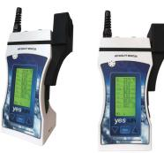
The YESAIR is available with an externally mounted particulate sensor for monitoring particulates in the air. The particulate sensor detects smoke, dust, pollen, spores, etc. particle concentrations in air by using an optical sensing method. A laser LED and a photosensor are optically arranged in the device and the photosensor detects the laser LED light reflected by dust particles in air.
