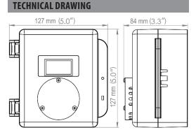
Note: Drawings above are shown with the optional splash guard. Without the splash guard, the thickness of the unit is 71 mm (2.8").
