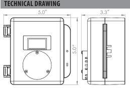
Note: Drawings above are shown with an optional splash guard. Without splash guard, thickness of unit is 71 mm (2.8").
