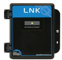
The LNK-XT Network Extender peripheral device works as a signal booster allowing transmission and receipt of gas readings over a larger total area. It extends the range of the Modbus® communication network allowing a longer distance between the Controller and the gas detectors. The micro controller quickly passes Modbus information packets from the master side of the LNK-XT to the extension side, seamlessly without interruption.
