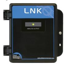
The LNK-AO Analog Output peripheral device adds four channels of 4 - 20 mA analog output to a Modbus® RS-485 network configured with a QCC Quad Channel Controller or an FCS Flexible Control System Controller. The LNK-AO is designed to send a 4 - 20 mA signal to up to four devices such as a data / trend / logging system, a BAS or DDC or up to four VFDs.
