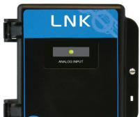
The LNK-AI Analog Input peripheral device adds four channels of 4 - 20 mA or 0 - 10 volt analog inputs to a Modbus® network configured with an FCS Flexible Control System Controller.
