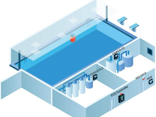
CGAS-D-CL2 transmitter should be mounted 6 inches above the floor
