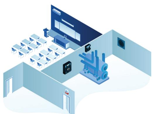
supplying the gas. Outside the room, above the door, there should be an audible/visual alarm device such as the RSA-24V Remote LED Strobe Light. If there are additional entrances to the room, each should have a remote visual/audible alarm device outside the door.
