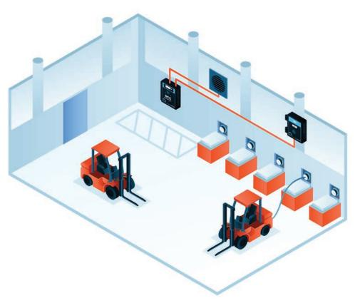
mounted on or near the ceiling above the battery charging area, where hydrogen gas will concentrate. Care should be taken to make sure the sensor is away from ventilation fans and any rapidly moving air.
