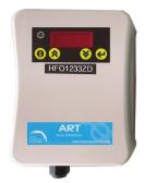
The ART gas detector is a state-of-the-art, fixed, nondispersive infrared refrigerant transmitter used to detect a wide range of refrigerant gases. The fast-responding sensor accurately detects refrigerant gas leaks without cross interference from combustible or toxic gases. It can be used as a stand alone system or integrated into a building management system (BMS).
