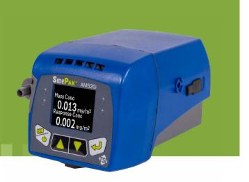
The SidePak™ AM520i Personal Aerosol Monitors are small, portable, battery-operated, data-logging, light-scattering laser photometers that provide real-time aerosol mass concentration readings of dusts, fumes, mists, smoke and fog within a worker breathing zone.
