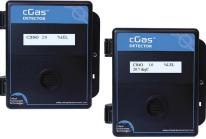
The cGas Detector Transmitter is a low maintenance gas monitoring device designed for use in non-explosion rated, commercial applications that require continuous monitoring of combustible alcohol gases and vapours such as methanol and ethanol. It offers one 4-20 mA analog output or a user selectable in the field digital output with your choice of BACnet® or Modbus® for communicating with a Building Automation System or ventilation controller.
