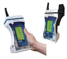
The YESAIR is a battery powered, portable air quality detection and data logging instrument designed for intermittent or continuous indoor air quality monitoring.
