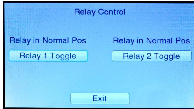
Figure 15. Relay Outputs screen in Diagnostics menu
