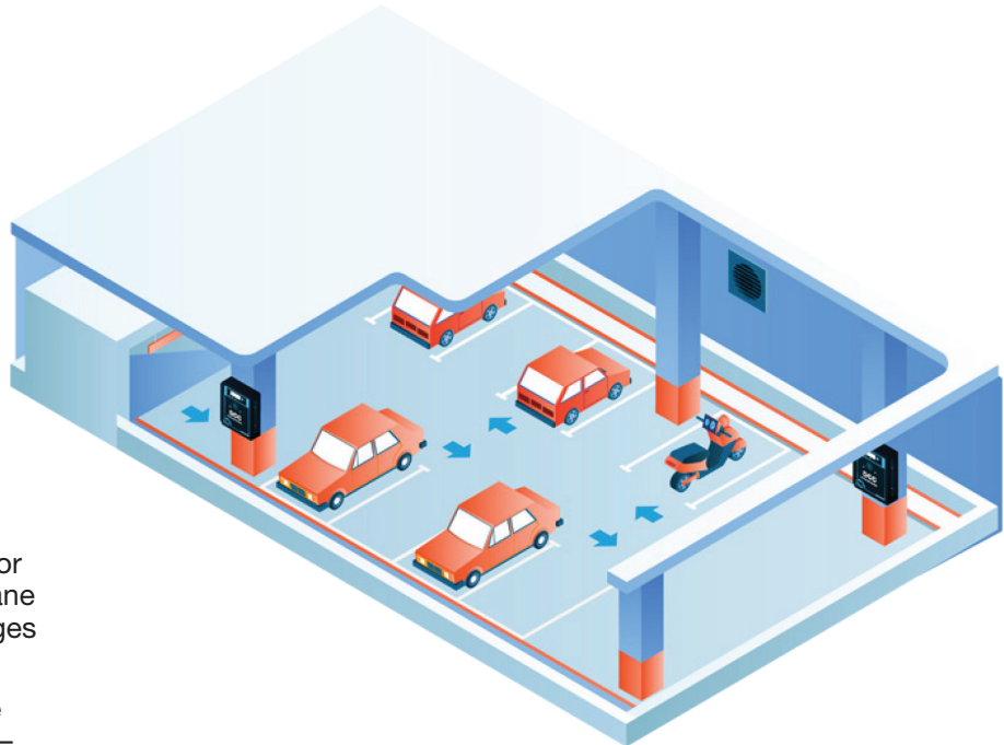
Example of continuous monitoring of vehicle exhaust in small to mid-size parking facilities; Source: CET Application Note
