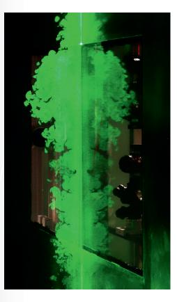
At the Institute of Fluid Mechanics and Aerodynamics of the Bundeswehr University Munich PIV measurements at large-scale structures are performed in the Atmospheric Wind Tunnel. The group around Prof. Kähler studies the fluid dynamics of large-scale structures in turbulent boundary layers.
