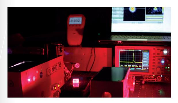
InnoLas succeeded in developing a high power 1319 nm laser with up to 800 mJ pulse energy. The laser is now available with two different resonator types (Multimode and VRM) to match different application requirements. Based on the field-proven SpitLight monolithic laser head design and components, it offers excellent long-term stability, same as any 1064 nm laser system.
