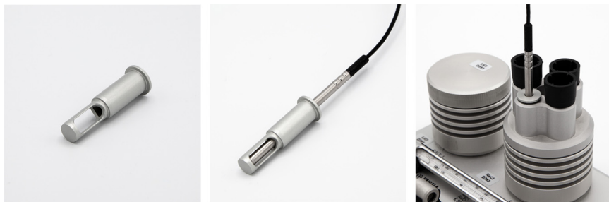
Figure 31 Using HMP9 calibration adapter with HMK15
