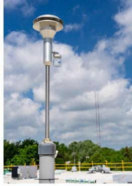
The Sampling System for Atmospheric Particles 3750200 is designed to sample and condition aerosol in preparation for measurement by the Condensation Particle Counter (CPC) 3750-CEN and by the Scanning Mobility Particle Sizer" (SMPS") 3938W50-CEN. The humidity and temperature sensor RHT3000 is installed at the inlet of the CPC 3750-CEN (or SMPS"); this sensor provides relative humidity and temperature data for the sample, as required by CEN/TS 16976:2016 and CEN/TS 17434.
