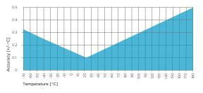
HMP7 Temperature Measurement Accuracy over Full Range
