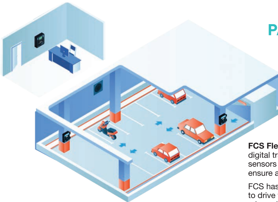
Example of continuous monitoring of vehicle exhaust in large enclosed parking facilities; Source: CET Application Note
