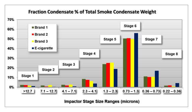
These results show how the Mini-MOUDI impactor enables determination of the aerosol mass contained in various particle size ranges. Further analysis of the samples collected on various Mini-MOUDI stages will reveal the distribution of chemicals, e.g., nicotine and tobacco-specific nitrosamines, in various size bins, providing valuable data concerning the access of the cigarette smoke contents to various regions of the smokers' lungs.
