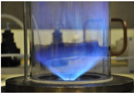
Flame diagnostics with PLIF (ERC, Laguna Hills, CA, USA)
