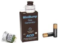
The MiniBump Test System is an ultra small, battery powered gas generator specifically designed for bump testing Chlorine, Hydrogen, Hydrogen cyanide and Hydrogen sulphide gas sensors.
