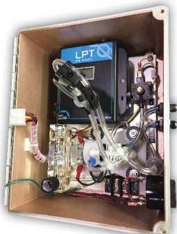
Inside of the DCC-MRI showing the LPT-A with Oxygen sensor.
