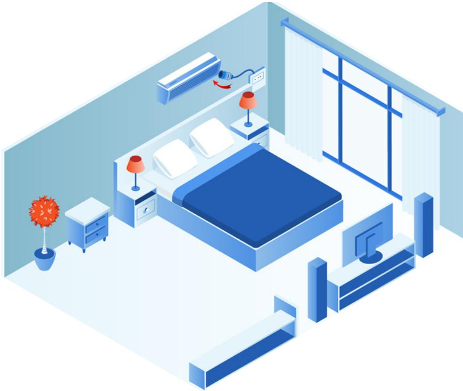
In packaged terminal air conditioner (PTAC) applications, the remote sensor model offers flexible placement options for the sensor, making it easier to place the sensor as close to the potential leak area as possible. The remote sensor should be mounted near the air conditioner coil and connected to the CGAS Detector with 18 awg wire stranded in conduit. The maximum length of wire between the remote sensor and the transmitter should not exceed 50 ft (15 m).
