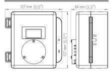
Note: Drawings above are shown with the optional splash guard. Without the splash quard, the thickness of the unit is 71 mm (2.8").
