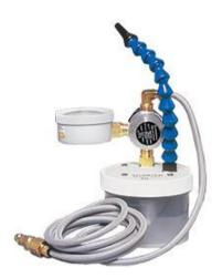
located in the jet-nozzle assembly. The jet creates an area of low pressure near the orifice which, in turn, causes the liquid in the reservoir to be sucked up into the orifice. The liquid is then broken into tiny liquid droplets and the compressed air carries the droplets through the outlet tube.
