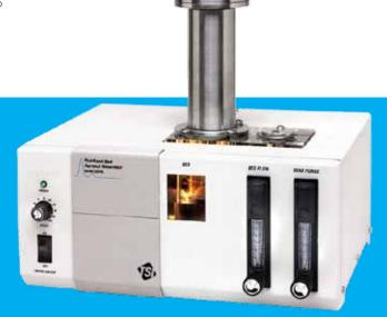
During operation, a bead chain meters powder into the fluidized bed. As air forces its way up through the screen and into the bed, it creates a boiling action, which deagglomerates the powder and causes it to be carried upward by the airflow through a vertical elutriator.
