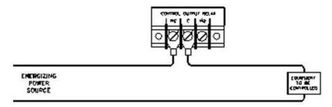
EQUIPMENT IS ENERGIZED FOR WIND SPEEDS BELOW THRESHOLD AND DE-ENERGIZED FOR WIND SPEEDS ABOVE THRESHOLD
