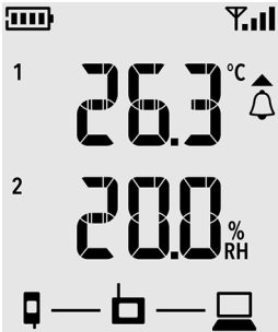
Figure 7 RFL100 with High Alarm Active on Channel 1
