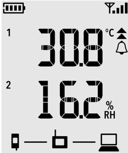
Figure 8 RFL100 with High-High Alarm Active on Channel 1
