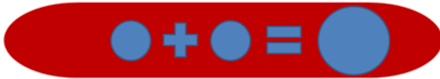
Fig 6 Particle coincidence, two particles in the laser beam
