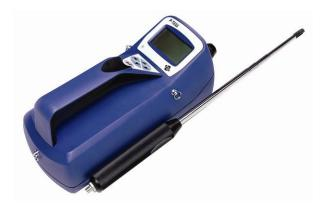
The P-Trak<sup>™</sup> Ultrafine Particle Counter uses fundamental measurement technology proven around the world in research and industrial applications since 1978. Its data logging feature allows the user to download field measurements for evaluation in TSI's TrakPro™ Data Analysis Software or in common word processing and spreadsheet programs, simplifying record keeping and reports.
