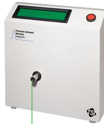
The PAM monitors monodisperse aerosol produced using a Model 3475 CMAG.
