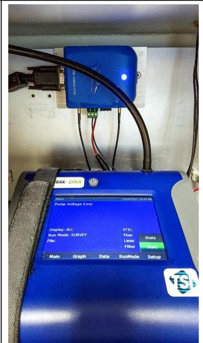
10. LED on the modem will blink while the modem searches for a network. If the LED stops blinking and is solid blue, a network has been found and proper communication with Environet should be possible. If the LED changes to solid yellow, the modem has not found a network. A power cycle may resolve the issue.
