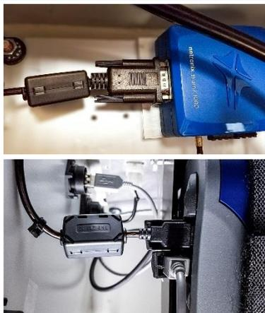
8. Finally, install the power cable as shown.
