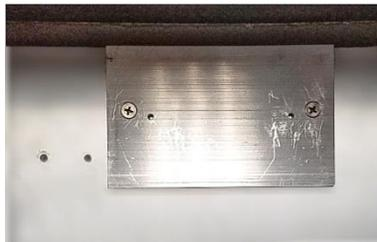
2. Remove the mounting plate from the back of the modem. To separate the two pieces, push the button on the top of the modem, rotate the plate slightly away and slide the mounting plate downwards.
