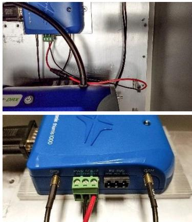
9. Plug the AC/DC power supply into an AC power source. Instrument and modem should power on.
