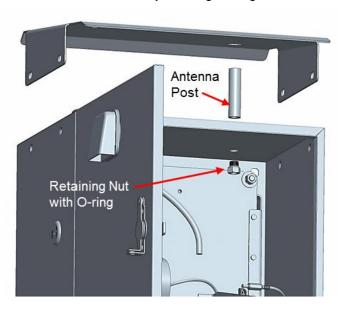
Using a 9/16" wrench attach heat shield, handles, washers, sealing washers, and nuts onto the enclosure as shown.
