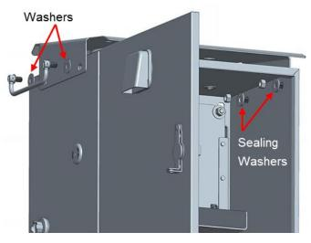
Before fully tightening the nuts install the Omnidirectional inlet. You may need to adjust the position of the heat shield.
